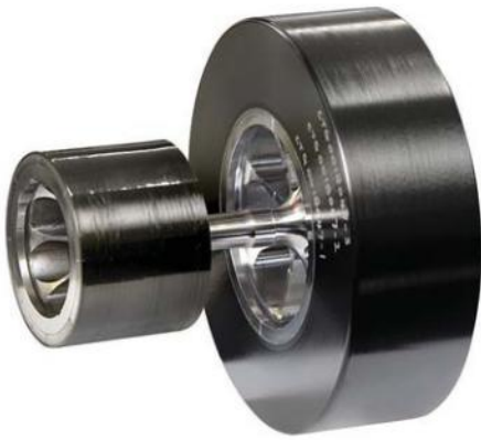
▲ Figure 3 A pair of flywheels with much of the mass distributed to be around the perimeter.
