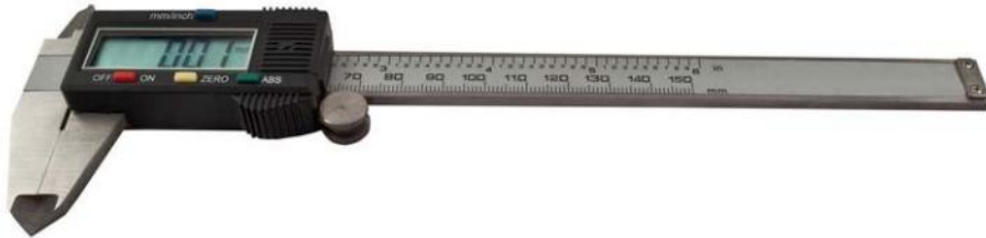
▲ Figure 1 Zero error on digital calliper.
